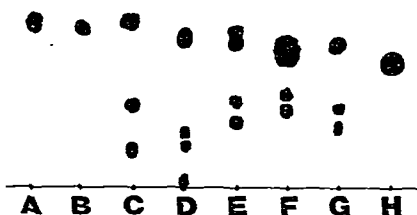
Fig. 1. TLC on silica gel. Solvent system, acetonitrile-water (9:1). A = 0.5 mg pentanone-2; B = 0.5 mg pentanone-3; C = 0.5 mg cyclobutanone; D = 0.5 mg cyclopentanone; E = 0.25 mg cyclohexanone; F = 0.25 mg 4-methylcyclohexanone; G = 0.25 mg 3-methylcyclohexanone; H = 0.25 mg octanone-2. Note: commercial products contained impurities.
